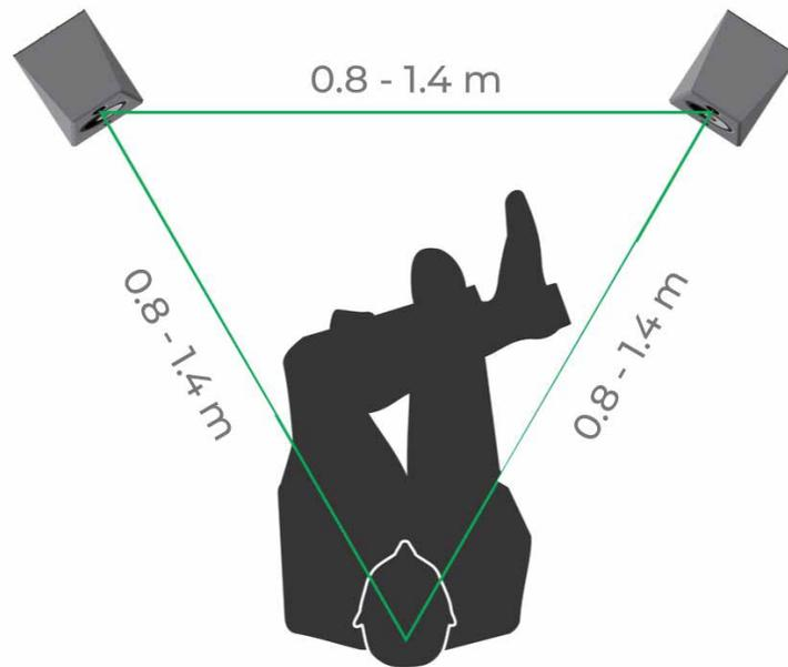
*A good rule of thumb to establish a solid stereo image is to construct an equilateral triangle between the two cabinets and the listening position.*
